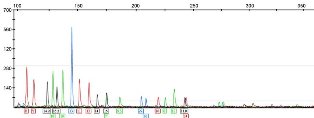
**Fig. 1.** An electropherogram (epg) showing several peaks close to the reporting threshold of 50 RFU (lower grey line). The highest peak, labelled 13, has no partner but since it is above the LTDNA threshold of 300 RFU (upper grey line) it is assumed to represent a 13,13 homozygote. In contrast, the genotypic designation 11,0 for a low peak allows the possibility of any other allele, including another 11, in the genotype of the contributor.
